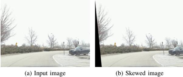
Fig. 6: An example of the skew we use to augment our dataset and use in our RL Simulator. Here, the skew is set to 0.1
