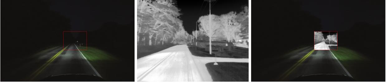
Fig. 2: Navigating in dark environments using RGB cameras can be challenging due to the lack of features. Thermal perception provides a truly passive approach to perception.
